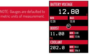
The items being monitored can be adjusted by pressing up or down on the device to highlight and then pressing the center button on the BDX to select which reading you'd like to change. Within this menu, you can change the item you're monitoring, and the units in which it will be displaying. You can also change the layout of the gauges within this menu.
